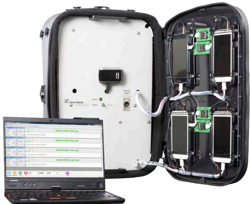
XGMA Smartphone as backpack version (right) and Android smartphone running MPSPM-a (left). Individual smartphones can be detached from the backpack for handheld measurement.
