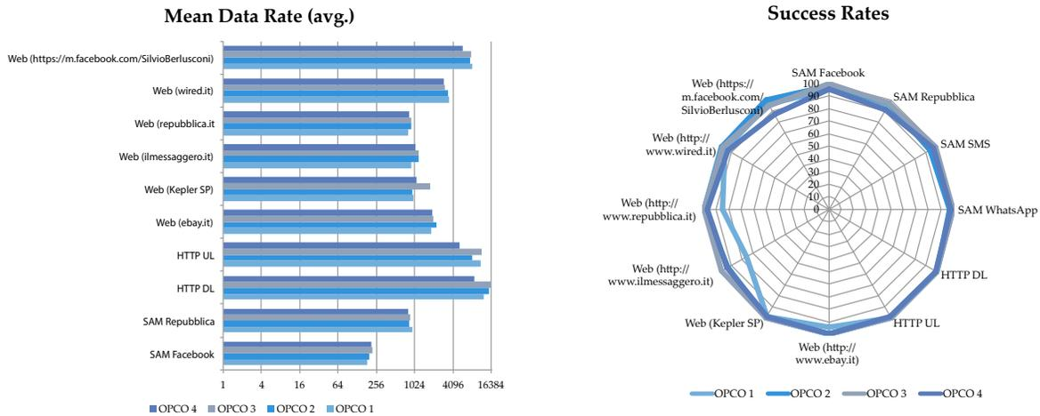
Example KPI diagram of SAM and conventional service tests from a benchmark test performed in Rome, Italy. On the left: Mean Data Rate. On the right: Success Rates-
